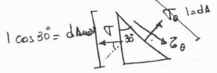
$$\sigma = \frac{2000}{A} = \frac{2000}{20 \times 10} \quad F_{\theta} = \sigma(1) \quad F_{2\theta} = \tau_{\theta}(1)$$
